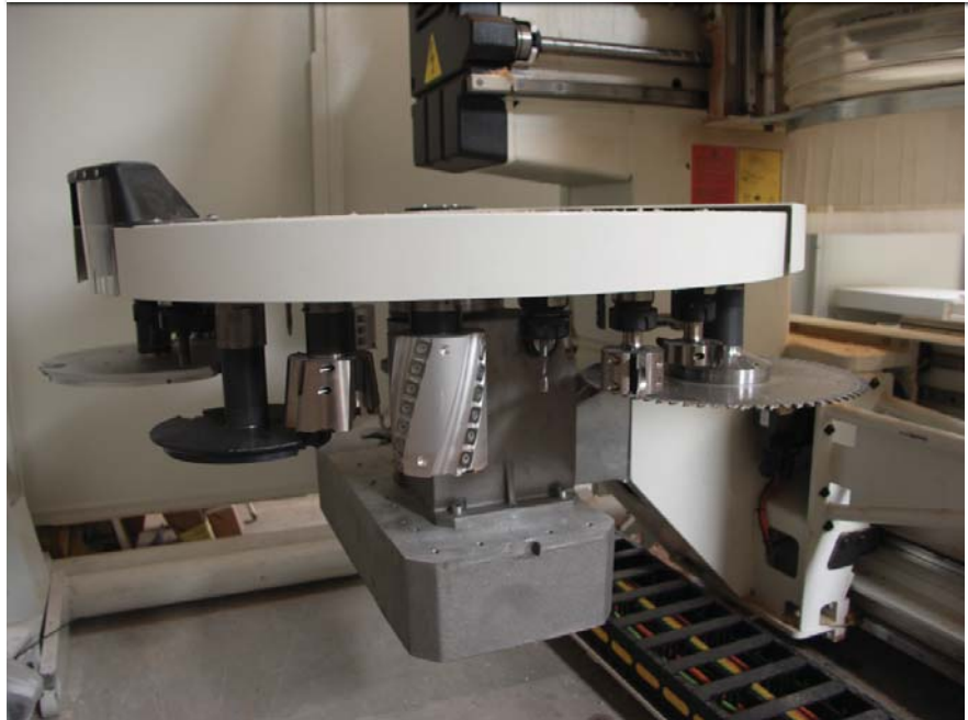
The SCM RAPID 24 tool changer on Cavendish Joinery's cnc machining centre
