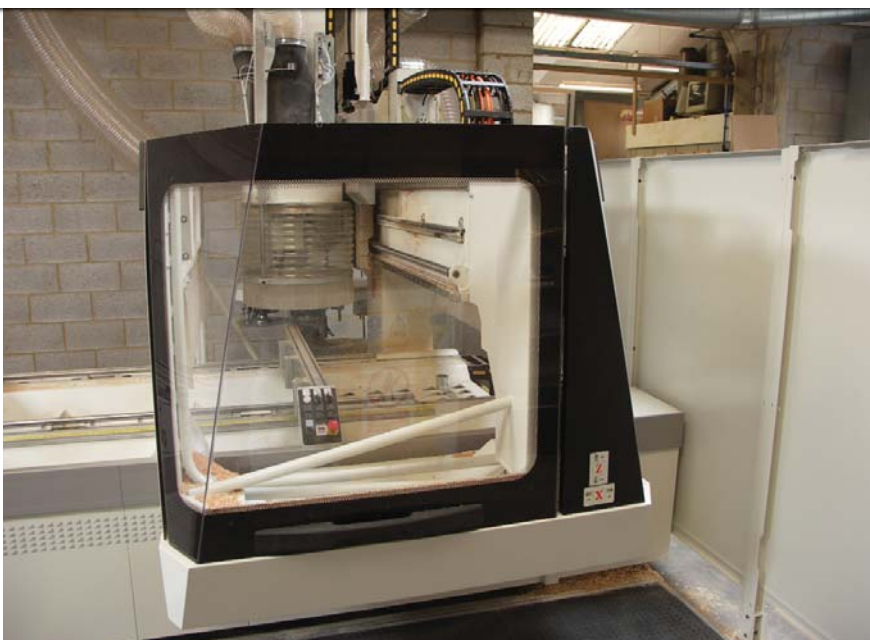
The PRISMA 5-axis machining head on the SCM cnc at Cavendish Joinery
