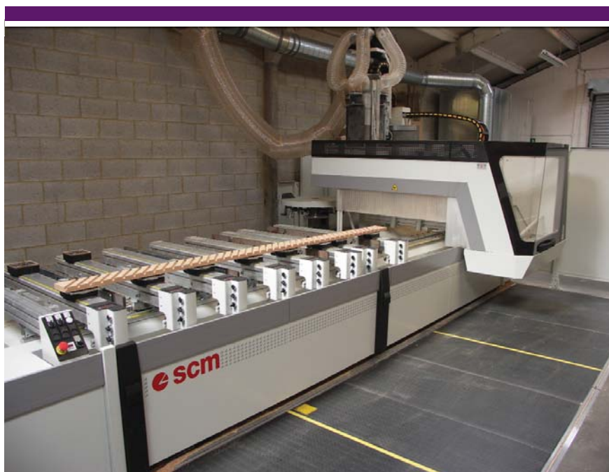
The SCM 5-axis cnc machining centre installed at Cavendish Joinery
